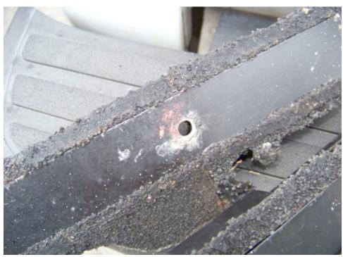
Leaks and corrosion found at point of penetration
