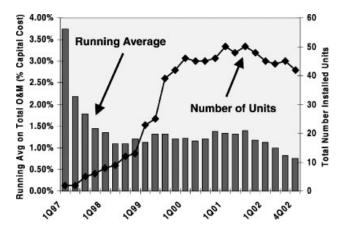
Figure 3. Running average of total quarterly O&M costs for OGR systems as a function of total number of installed systems
