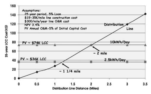
Figure 7. OGR LCC versus line extension LCC
