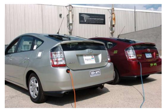
Plug-in vehicles, such as these plug-in hybrids, can contribute to stabilizing the grid by providing electricity storage capacity. Energy storage is a key technology that can enable renewable sources of energy such as solar energy to plat a larger role in America's energy fut@ecdit: Argonne National Laboratory
